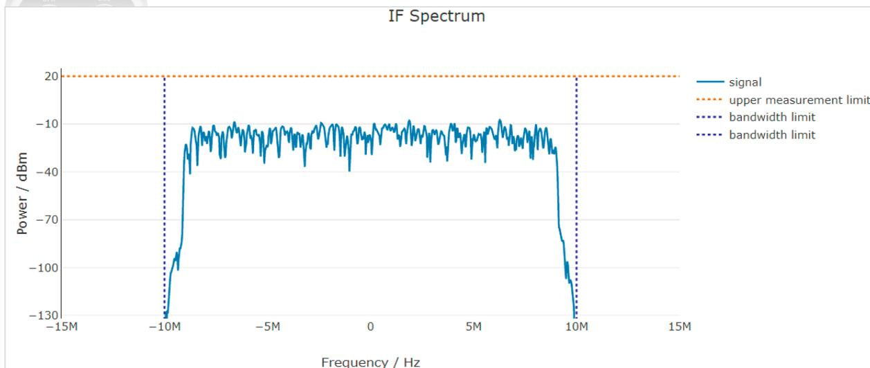
Signal check for a 20 MHz LTE signal.
