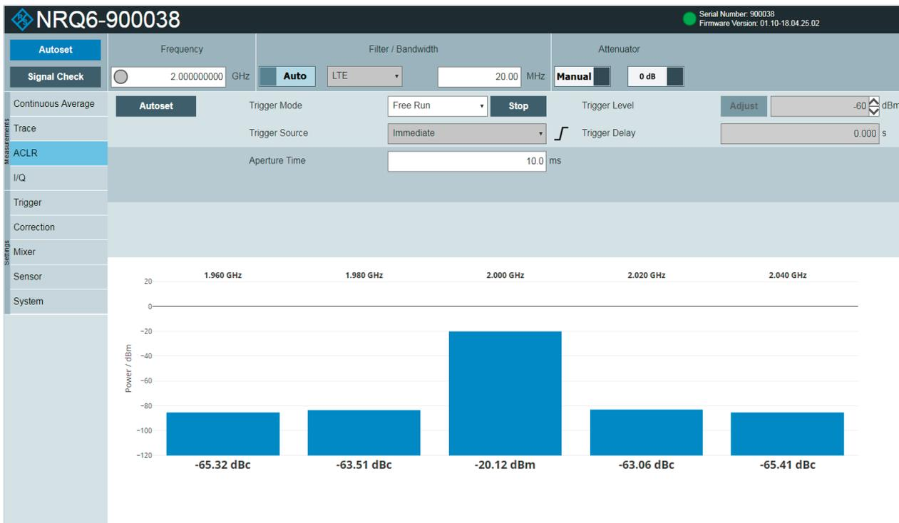
ACLR measurement on a 3.84 MHz 3GPP signal.
